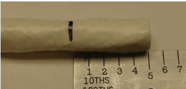
Figure 11: Marking the cable
