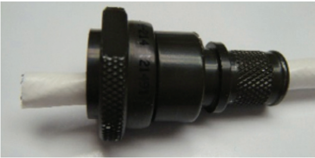
Figure 42: Inserting backshell on the cable
